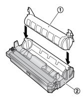
**8** Firmly press down the toner cartridge to snap into position.
